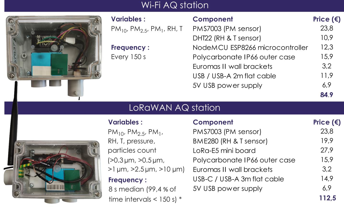
\* According to ESTI regulation, the measurement period is adapted to the datarate depending on the range between the LoRaWAN AQ station & the gateways (5 to 160 s).
